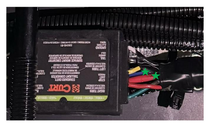
6. Cut the remaining wires on both sides of the NEW tail light converter box, ensuring that you leave approximately 3" of wire to reconnect to the wires on the chassis.
