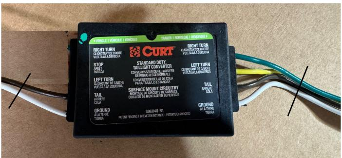
NOTE: DO NOT CUT THE 10G RED WIRE AND 14G BLUE WIRE THAT ARE IN THIS SAME GROUP OF WIRES, THESE ARE FOR THE BRAKE CONTROLLER AND POWER.
