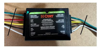
**7.** Using the 22-18 G Butt Connectors and torch lighter, connect each chassis wire to the matching wire color of the new tail light converter box, ensuring that the vehicle side and trailer side do not become switched.
